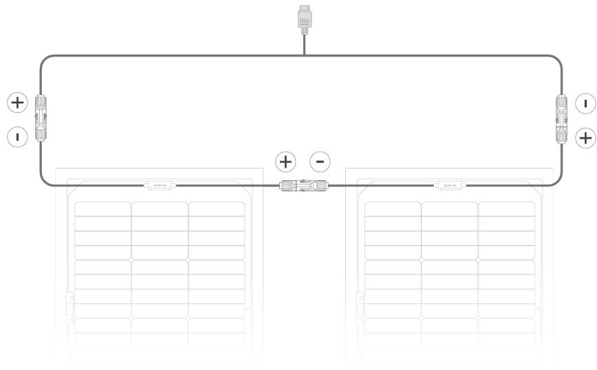
To wire **in parallel**, connect all positive ends of the panels' output cables to a [solar parallel connection cable](#), and do the same for the negative ends. Then, connect the [solar to XT60i charging cable](#) to the solar parallel connection cables. When connecting, refer to the instruction images to avoid misconnecting the male and female connectors of the parallel connection cables.
